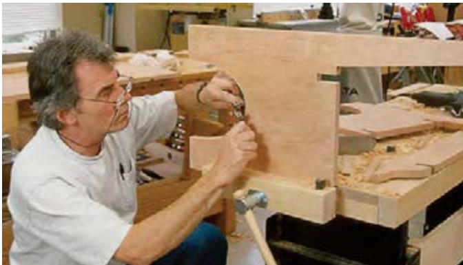
A spokeshave eases the edges the block plane couldn't reach.
