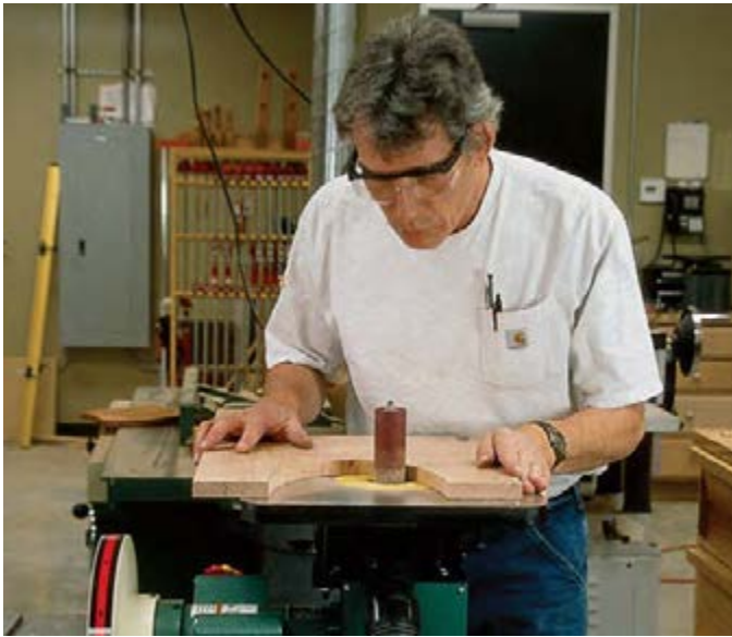
The oscillating spindle sander is ideal for cleaning up the saw marks and sanding to the inside of the pencil line.
