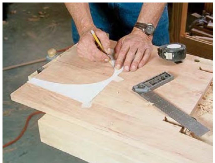
After the joints are cut and the back extension is glued on, position the paper pattern and mark the arched cutout.
