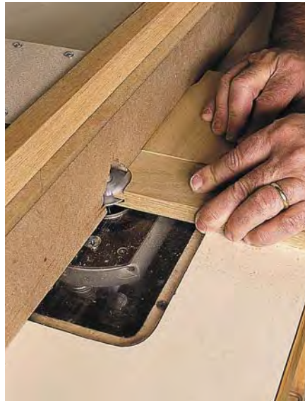
Use a block of scrap to push the end of the rail into the cutter for the cope. It will prevent tear-out and give you better control.
