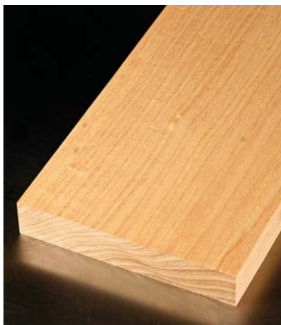
Lumber can't read. Most pieces of wood will have a combination of grain patterns, with a different appearance on one side of the face than the other.
