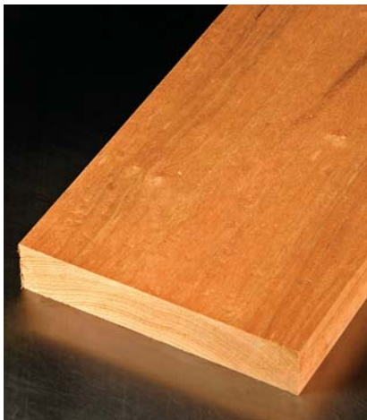
Plain-sawn. Growth rings that arch across the end of a board create "cathedral" shapes on the face of the board. While attractive, plain-sawn lumber is most likely to cup or twist.
