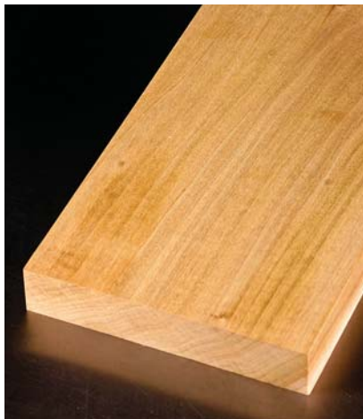
Rift-sawn. The growth rings slant across the end of rift-sawn lumber. The grain pattern on the faces and edges is straight and this cut is stable.
