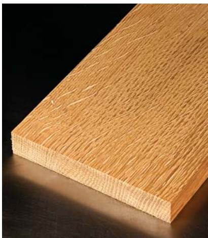
Quartersawn. The growth rings in quarter-sawn lumber are vertical, or nearly so. This type of wood will move more in thickness than in width.
