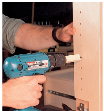
Use a stop collar on your drill bit when drilling holes for the shelf pins. I made this drilling jig from shop scrap.
